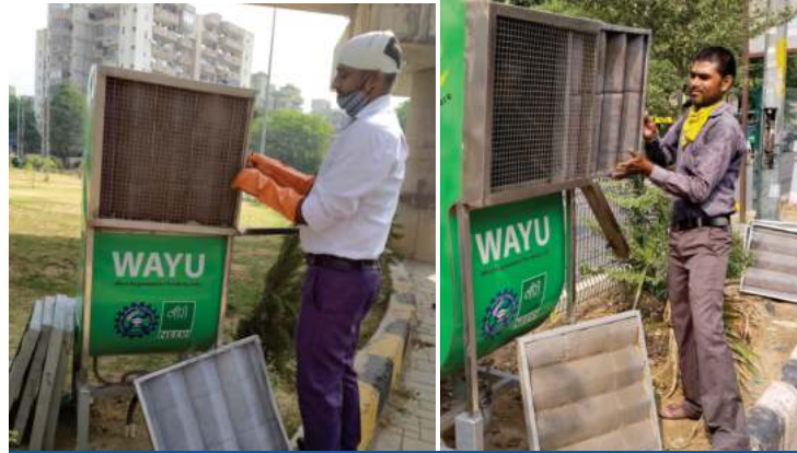
Operation & Maintenance of WAYU Purifiers and Installation of Air Quality Monitors Under Project PAC
