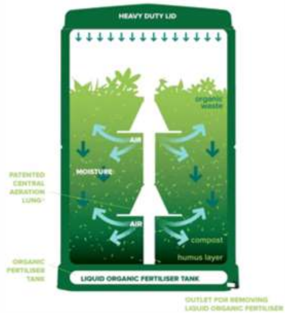
Figure: Functional Design of Aerobin
