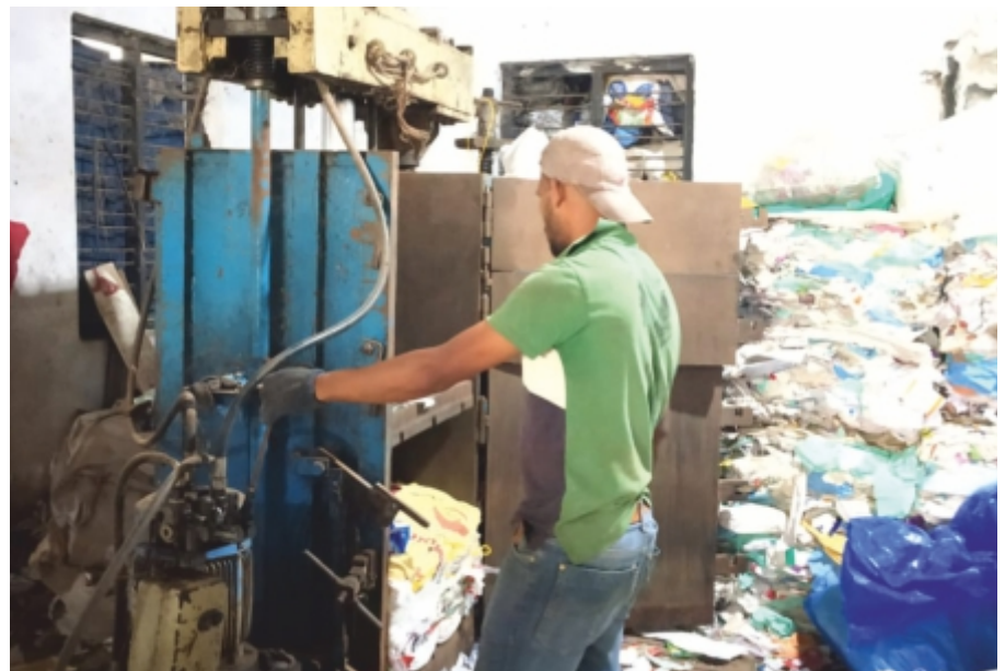
Figure 6: Bailing process at the dry waste collection centres
